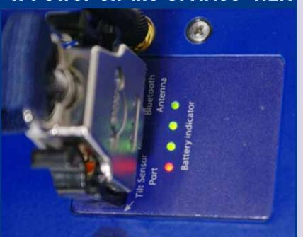
Plug in the ON/OFF Dongle to turn on the SPAA05-NEX tool.
