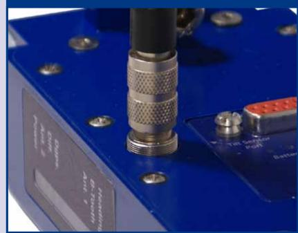
Plug in the tilt sensor connector to power on the tilt sensor.
