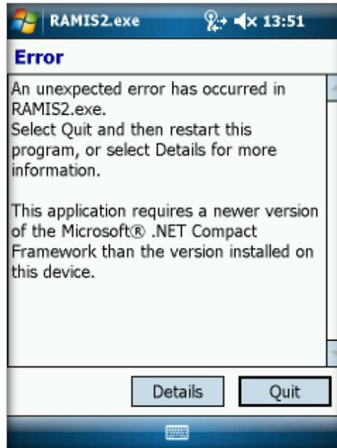
**A: RAMIS** is a **.NET Framework** build program and you will need to have at least **.NET Framework 3.5** installed on your PDA. The installation file can be freely attained from Microsoft. You can find information on how to install .NET Framework in **subsection 2.1.2**.
